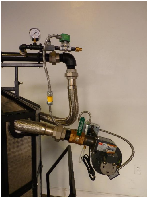
If your furnace comes with the Air Preheat hose, it is recommended that it is engaged for your initial firing. The Preheat hose creates drag on the air flow, which allows for a slower heat-up.
