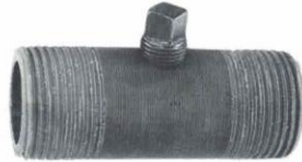
INSULATING/PURGING NIPPLE (Phenolic) Reduces conducted heat. When used with regulated purging air it also reduces convected heat. Supplied with \frac{1}{8} " N.P.T. tapped hole and plug to receive purge air connection.
